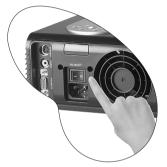
3. Press and hold POWER for 1 second to start the projector. The back-lit POWER key flashes green and stays green when the power is turned on.
