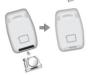
Avoid excessive heat and humidity. There may be danger of an explosion if batteries are incorrectly replaced. Replace only with the same or equivalent type recommended by the manufacturer. Dispose of used batteries according to the manufacturer's instructions.
