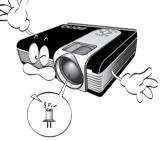
Never replace lamp assembly or any electronic components unless the projector is unplugged.
